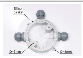
Connection box mounting holes (2 x 5 mm) c/c = 108 mm. The connection box is prepared for required number of compression glands, two (in / out) or three (in / out / ext. LED). A gland is approx. 30 mm high.
